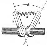
FIG. 133. dynamometer illustrating the principle of the synchronous motor.
